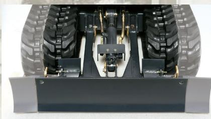
With the simple removal of one pin, its quick-fold blade adjusts in size instantly.
